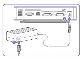
Connect the power cable to the DC power adapter. Connect the DC power adapter to [DC 14V] on the product.
